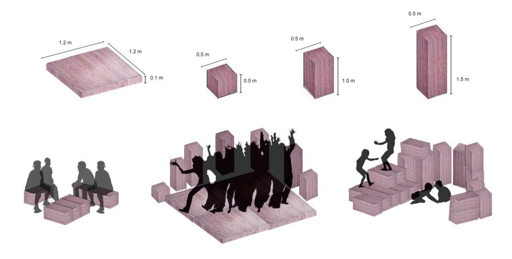
The forms are simple, moveable and are constructed from locally harvested cedar plywood to reflect the history of logging and native species of Burnaby. The forms are a platform, for dance parties, that also defines the ground plane; the seat; table; a leaner or screen that could be used to create privacy or enclosure, or could be used to build forts or theatre sets. The forms could also be lit from within to act as wayfinding devices and icons in the alley.
